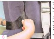
3 Pull the vehicle belt out, then pass the vehicle belt through the first belt slot, from the front of the restraint to the rear (*Fig. B*).
